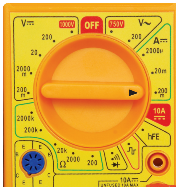
Figure 5-6. The meter dial at the 200m position to measure current.
